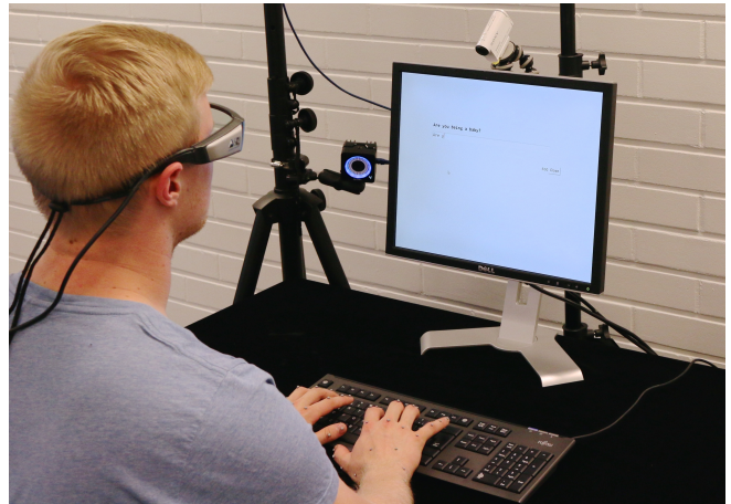
Figure 2. Experimental setup: The typing process of 30 participants was captured using a motion capture system and eye tracking glasses. In addition, keypress timings were logged and a reference video recorded.
